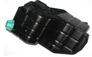
İMBUSAT DEPOSU ACT. EXPANSION TANK
